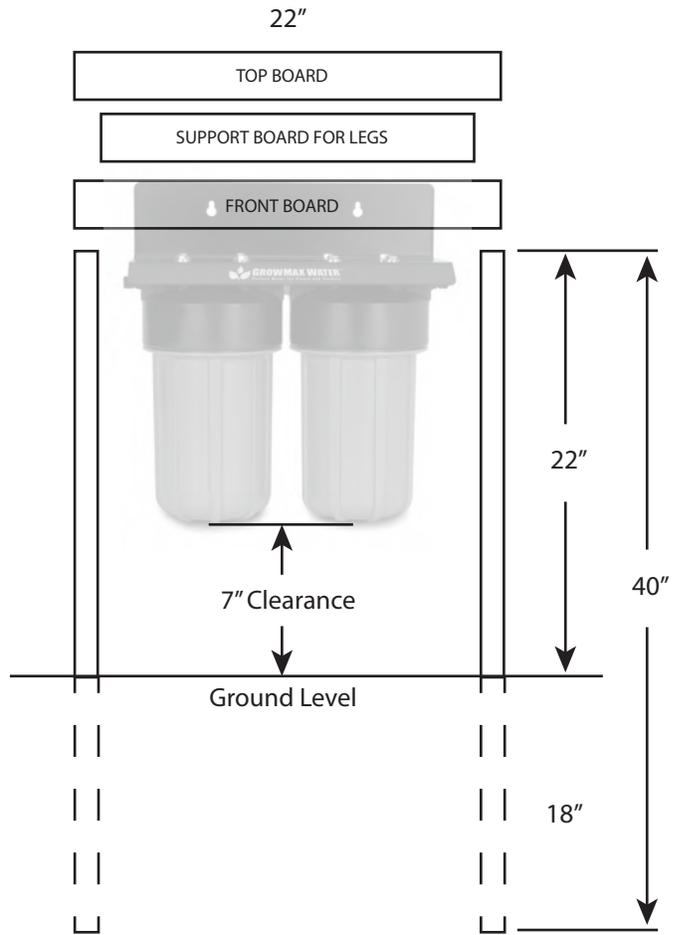
Mount unit using large 2" wood screws
